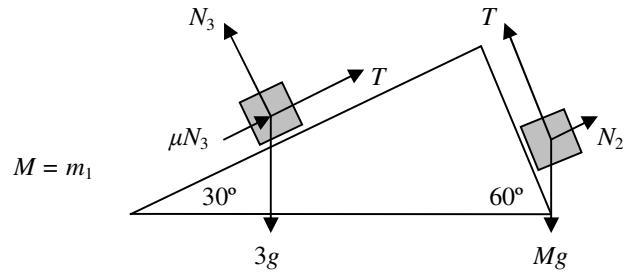
$$3\text{-kg mass: } 3g \sin 30^\circ - \mu N_3 - T = 0, \quad 13.427 - T = 0 \quad \dots \quad (1)$$
