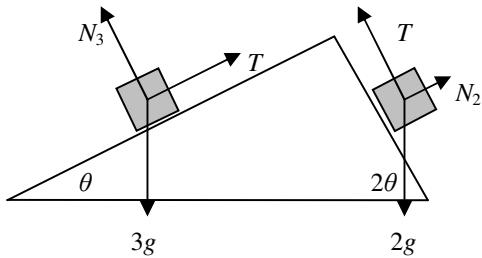
$$Q4a \quad T - 3g \sin \theta = 3a \quad \dots \quad (1)$$
