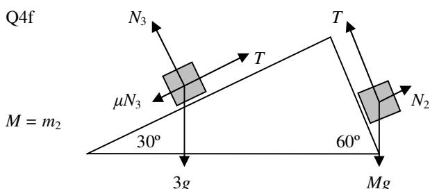
$$3\text{-kg mass: } T - 3g \sin 30^\circ - \mu N_3 = 0, \quad T - 15.97306 = 0 \quad \dots \quad (1)$$
