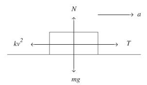
The train's equation of motion in the horizontal direction is  $T - kv^2 = ma$ .
