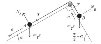
Particle A: normal reaction force  $N_A$ ; weight force  $m_1g$ ; tension T
