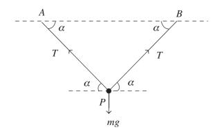
Resolving forces in the vertical direction we have  $T\sin(\alpha) + T\sin(\alpha) = mg$ .
