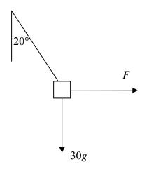
The magnitude of the horizontal force, *F* newtons, required to hold a 30 kilogram child in equilibrium on a swinging rope, as shown in the diagram above, is
