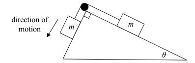
Two bodies each of mass, m kg, are connected on a back-to-back plane by a light string passing over a smooth pulley, as shown in the diagram. The coefficient of friction of the surface of each plane is  $\mu$ .
