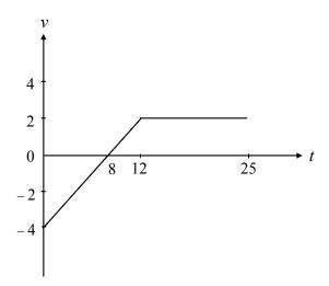
How many metres is the particle from its starting point after 25 s?
