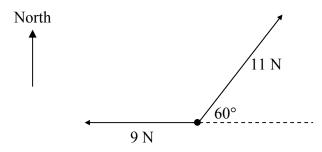
Correct to the nearest degree, the resultant force acting in an anticlockwise direction from due east will be
