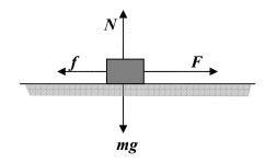
A body of mass m kg is pulled along a rough, horizontal ground by a horizontal force F newtons as shown above. If N is the normal reaction, f is the force of friction and  $\mu$  is the coefficient of friction, which one of the following statements is true?
