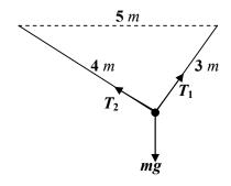
A particle of mass m kg is supported by two strings of lengths 3 m and 4 m as shown above. The other ends of the two strings are fixed at two points 5 m apart on the same horizontal level. If tensions in the strings are  $T_1$  and  $T_2$  newtons, which one of the following statements is true?
