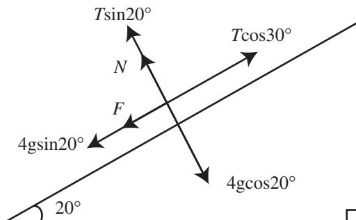
Forces shown on the diagram have been resolved parallel and perpendicular to the plane.
