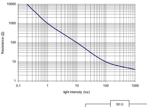
The LDR is placed in a circuit on the right.
