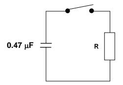
When the switch closes it takes 2.35 seconds to fully discharge the capacitor. What is the size of the resistor?
