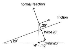
As seen in the diagram the friction force = sine component of the weight force, since the speed is constant. So,
