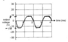
The output varied about zero, was inverted, had the same frequency as the original and was clipped at +8 and -12 V.
