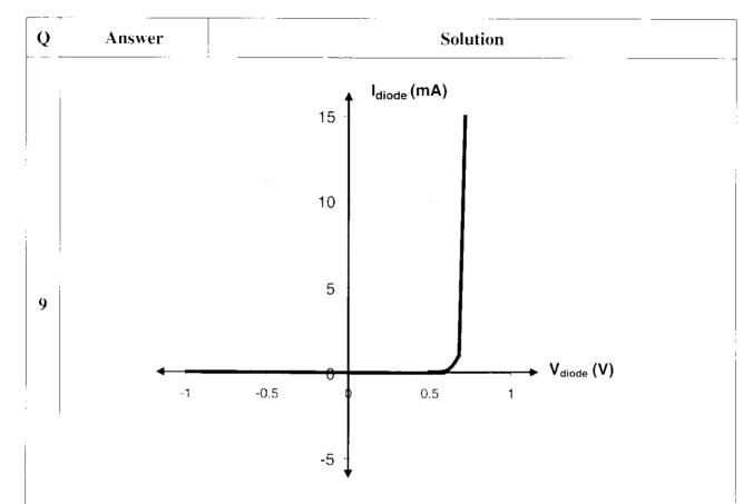
Line follows the x-axis from the left until about 0.7 V where it curves upwards indicating that the diode starts conducting when this voltage is applied across it.
