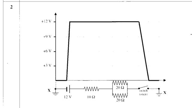
The switch is open, so no current flows in the circuit so there is no potential difference across the resistors. The whole 12 V drops across the switch.
