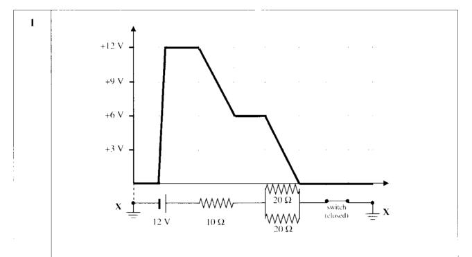
The two 20  $\Omega$  resistors in parallel are equivalent to a single 10  $\Omega$  resistor,  $\therefore$  the potential difference will be 6 V across the single 10  $\Omega$  resistor and 6 V across the parallel combination.
