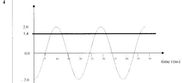
The diode will use 0.6 - 0.7 V which decreases the peak voltage to 1.3 - 1.4 volts. The capacitor will smooth the half wave rectified voltage to a virtually flat line due to the long time constant (3.3 s) compared to the period of the input signal (0.02 s).
