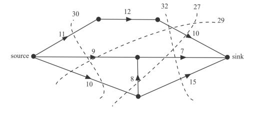
The minimum cut of 27 gives us the maximum flow possible through the network. Note that the pipe with a capacity of 8 L/min, flows from the sink side of the cut whereby it should flow from the source side to the sink side and hence we ignore this capacity of 8 L/min.
