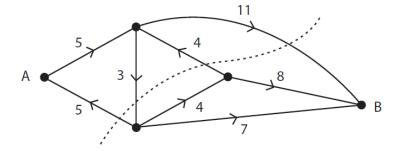
Considering the flow from A to B, the capacity of the cut shown in the network is **A.** 7
