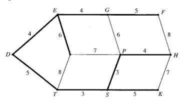
The minimal spanning tree is shown above. Nine edges form the minimal spanning tree.
