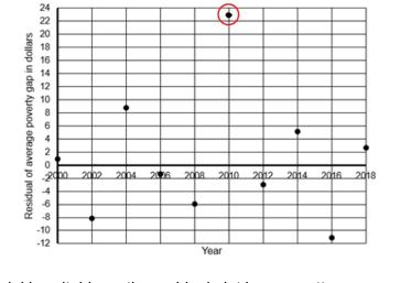
The linear model is suitable as the residual plot has no pattern g. (is randomly scattered).
