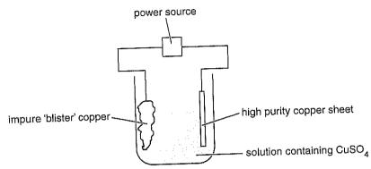
In this electrorefining process the 'anodic mud' which collects under the anode is recovered.
