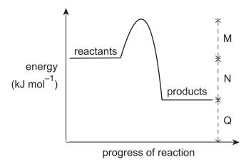
For the forward reaction, the enthalpy of the products is 50 kJ mol<sup>-1</sup>, the activation energy,  $E_a$ , is 30 kJ mol<sup>-1</sup>, and the enthalpy change,  $\Delta H$ , is –60 kJ mol<sup>-1</sup>.
