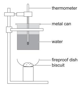
In the experiment, one biscuit was weighed, placed in the fireproof dish and ignited. After the biscuit finished burning, the remains were allowed to cool and were then reweighed. The temperature of the water in the metal can was recorded before the biscuit was ignited. The highest temperature that the water reached after heating was also recorded.
