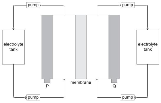
Different vanadium-based chemicals are stored in each electrolyte tank and pumped into the cell to produce electrical energy via a chemical reaction that occurs according to the following equation.
