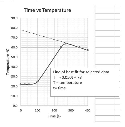
50.0 mL of 1.00 M copper(II) sulfate was placed in a polystyrene cup and zinc powder was added **after 60 seconds**. The temperature data was obtained using a data-logger. The graph above shows a plot of the data. A dotted straight line has been drawn through some of the data points. The equation for the line given by the data logging software was T = -0.050t + 78
