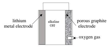
The overall equation for this cell is shown below.
