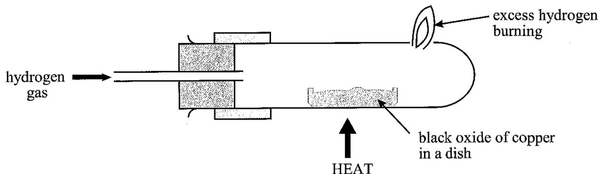
After heating, the stream of hydrogen gas was maintained until the apparatus had cooled.
