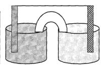
Zinc electrode in an aqueous zinc nitrate solution
